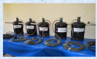
Detail experiment was set up for the production biogas using different combinations of press mud, cow dung /
