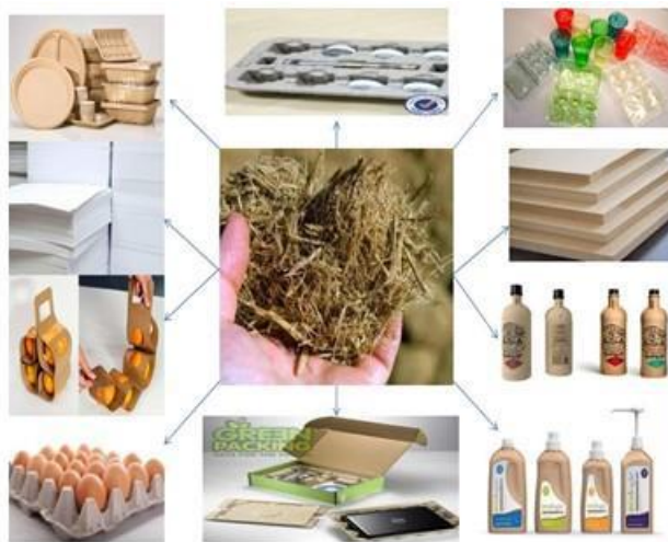
Fig 3 (a) Multiple bagasse products: - tableware, paper, packaging, bottles, MDF board, plastic composite resins
