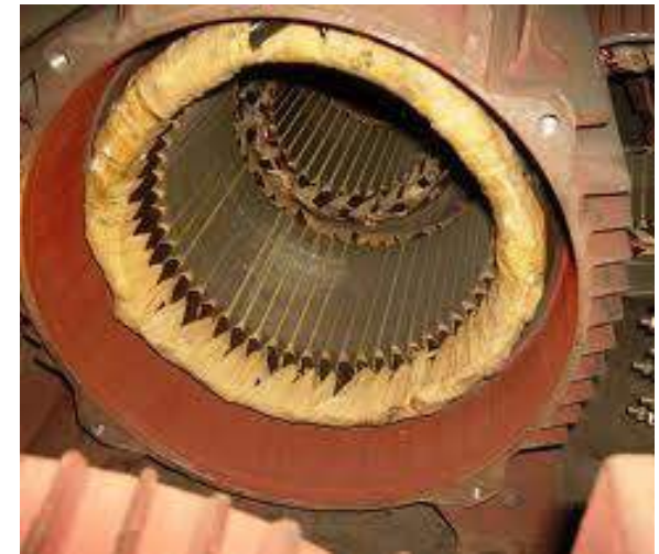
stator core with ribbed yoke
