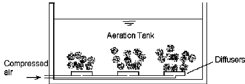
Figure 19.2. Typical air diffusers arrangement
